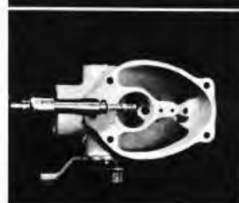
28— Install Main Nozzle and Gasket.
