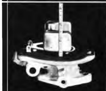
24— Install Float and Lever Assembly and Float Lever Pin. Set floats \frac{1}{4} " from gasket face to nearest edge of float, keeping edge of float parallel with gasket. Adjust by using bending tool #M-8.
