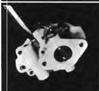
21— Install Idle Adjusting Needle and Spring. Set approximately one turn from seat for preliminary setting.
